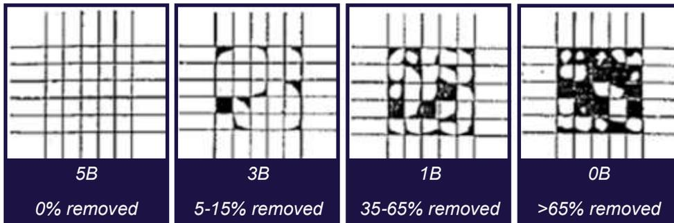
Example: UltraGrip WB 7000 Primer Adhesion Testing Results
